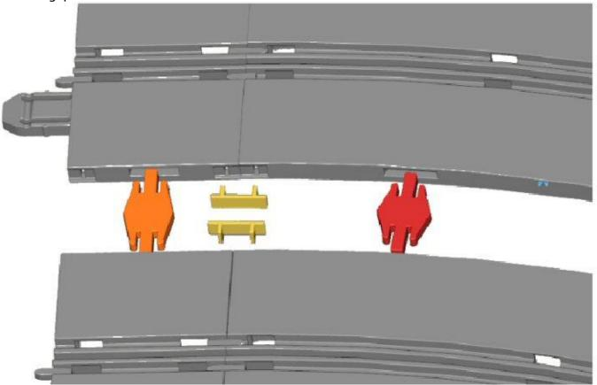
They have designed the geometry, so that a layout can have the turns altered, while retaining the main structure, as the geometry of the various curves simply requires the addition or subtraction of half straight pieces to restore continuity.
