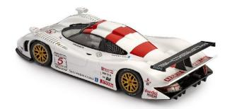
Chassis: Podded Motor: Slot.it Flat-6 20,500rpm, 200 g/cm torque 10.25 watts @ 12v dc (Mn09h) mounted as angle-winder with 1.0mm offset Axle & Gears - 2.38mm (3/32nd) Gearing: Crown 28t (GA1628-pl) - Pinion 11t brass Has adjustable height front axle - requires optional M2.0 Hex screws, not supplied with car Hubs Front: plastic 17.3mm x 8mm Hubs Rear: alloy 17.3mm x 8mm Tyres front: Product code PT1159C1 Tyres rear: Product code PT1167C1
