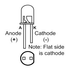
Another way to tell which is the negative side of your LED is to look for the small "flat" on the base of the LED head. This is always on the negative side of the LED
