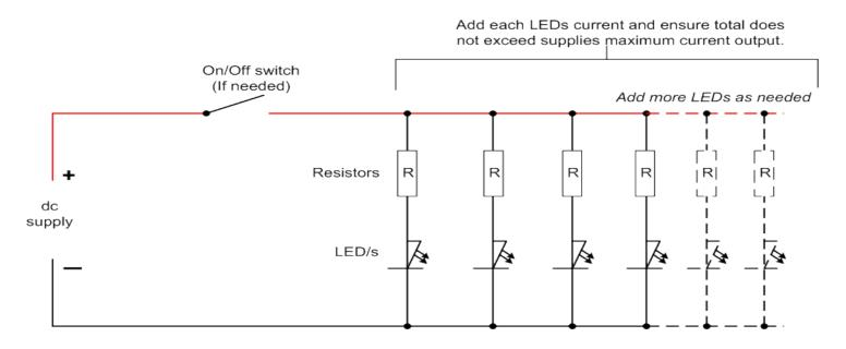
That should be sufficient to get the average beginner working happily with wiring LED circuits
