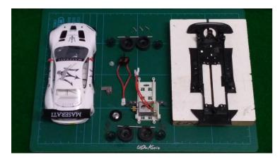
When you turn the body upside-down, you notice a shallow cockpit, which avoids interference from the rear cables (which pass over the motor) and from the central connector. The cockpit is an "interlocking solution" (no glue, no soldered parts), a pleasant solution already encountered in the DTM Slot.it, useful for easy cleaning and / or replacing it with a lexan one to decrease the weight.
