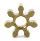
7 tooth and 8 tooth M50 (about 48 pitch) pinions to enable lower gearing on these low torque motors, for better braking.
