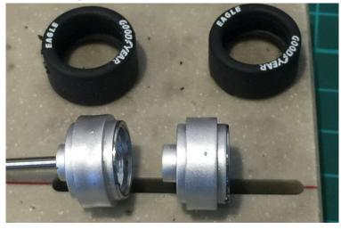
These are a tight press fit on the axle, twist carefully and pull off straight, so you don't risk cracking them. Plastic wheels are injection molded and can sometimes have small burrs. See above the small imperfections on both wheels. These ones weren't bad, but I still scraped them with a sharp blade, then sanded smooth.
