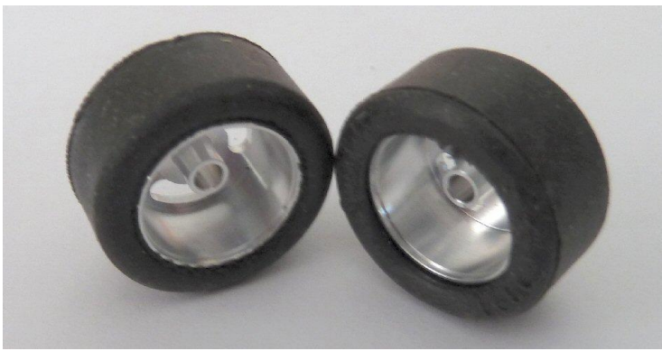
Left - wide shoulder inside Right - Wide shoulder overhanging
