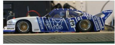
Having raised the rear axle with the replacement axle mount, and trued down the replacement tyres so they are slightly smaller OD than the originals. The ride height is greatly lowered. The back is about 1.3mm lower.
