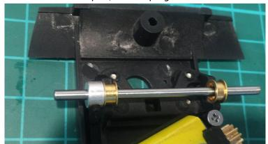
Now you can sit the axle and bushes on top of it with the concave side of the bushes to the inside, so the load bearing surfaces are as wide as possible for axle stability. Press gently on both sides at once, until the bushes click down into the new axle mount.
