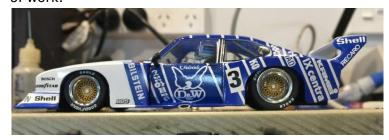
So here is the car unboxed. Take a look at the ride height as it comes. About 2mm of ground clearance front and rear. We will drop that, to lower the centre of gravity.
