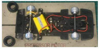
The mechanics are mostly Slot.it parts, axles, wheels, motor and gears. The fronts are  $15.8 \times 8$ mm plastics, the rear are  $17.3 \times 8$ mm alloy.
