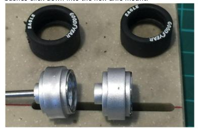
Now we can go to work on the fronts. These are a tight press fit on the axle, twist carefully and pull off straight, so you don't risk cracking them.
