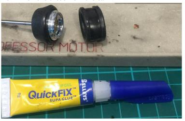
But first, let's get some race tyres fitted for wood racing Above are a pair of Slot.it PT1172N22 tyres, which will fit any hub from 15.8mm diameter, to these 17.3mm hubs.
