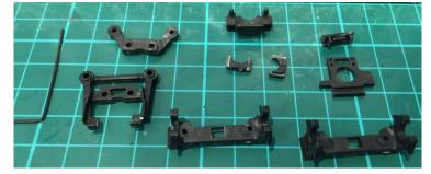
Make sure you look underneath the base, there is a hex key, and a pile of small plastic bits for adapting the ride height, and for swapping out the Slot.it Flat-6, for an FK180 "boxer motor of any brand. Front right are two axle mount brackets that will take axle bushes. If you look closely they are marked with lettering. One of which reads 0.5 and the other 1.0
