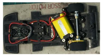
You could of course neatly cut some sticky back lead to fit the forward area, but I was out of it, and I am a bit impatient. So I have fitted a small half circle of cardboard in an arc, part filled the entire area in front of it with JB KWIK – the 10 minute cure version of JB WELD, and poured lead buckshot over it, then topped with a little icing of more JB KWIK as it sets. – No, I don't know the weight, but at a guess, around 9 grams.
