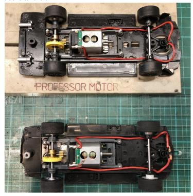
Standard chassis top, and after trimming donor chassis at bottom Test fit. Looks okay, but the whole front is sitting 1.5mm clear of
