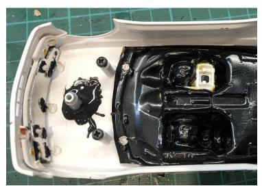
I then screwed it up tight through the chassis, roughed up the inside of the body shell for the epoxy, laid a generous amount on the body, some onto the post, and just left the car sitting upside down, so epoxy could slide down the body post and meld with that on the chassis.
