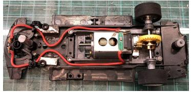
Plan B was mounting two rectangular plastic blocks against the chassis rails, and glue a soft rubber spacer onto the top of each, aligned to the body posts. I then screwed a body screw into each post, until the body sat at about the right height, with the screw heads sitting on the rubber spacers.
