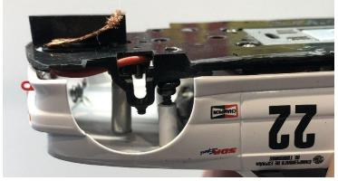
Having achieved this approximate ride height, I made a body post by using some soft plastic tube with an inside diameter a bit under 2mm, and epoxyed it inside some aluminium tube for strength and greater surface area for later fixing. I made the inner plastic shaft a bit longer than the aluminium tube, so I could trim the plastic to fine adjust the post length. You can see the silver aluminium shaft I the picture above, just about touching the inside of the bonnet.
