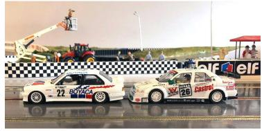
Rolling car, sitting on track with a Slot.it Alfa 155. As you can see I have clearly achieved a ride height several mm lower than the Alfa. This lower COG helps the handling, and even though track is still 1mm narrower than the narrowest of the Slot.it models, - the CA35 Castrol and Jagermeister liveries, it actually runs very well without having added any additional weight. But I will play around with this over the next few days for optimal lap times and predictability when pushed to the limit.
